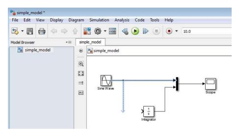
**3** With the cursor at the end of the dotted red line, move the cursor so that it lines up with the light blue guide arrow that points in the direction of the Integrator input port. The cursor turns into a hollow arrow.
