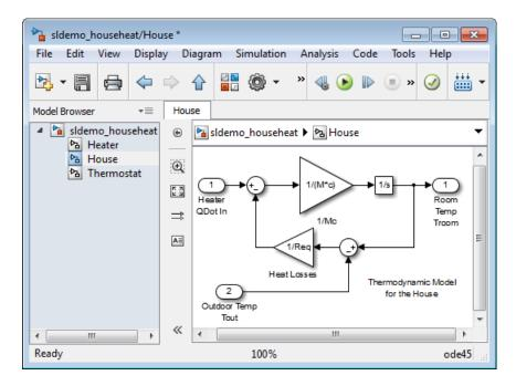
The House subsystem receives heat flow and external temperature as inputs, which it uses to compute the current room temperature. You could leave each of these blocks at the top level of the main sldemo househeat model, but combining them as a subsystem helps to simplify the block diagram.
