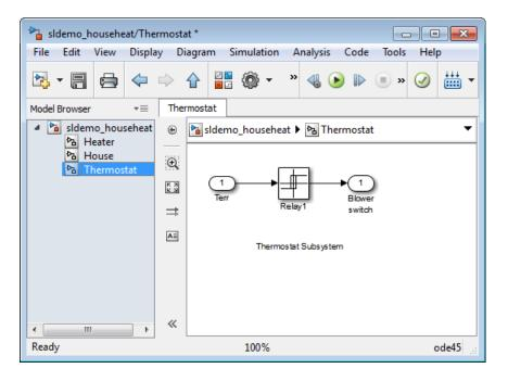
This subsystem models the operation of a thermostat, determining when the heating system is on or off. It contains only one Relay block, but logically represents the thermostat in the block diagram.
