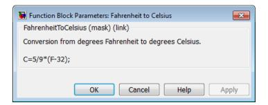
3 To view the underlying blocks in the Fahrenheit to Celsius conversion subsystem, select the Fahrenheit to Celsius Subsystem block and then select Diagram > Mask > Look Under Mask.
