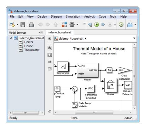
**2** Subsystems can be complex and contain many blocks that might otherwise clutter a diagram. For example, to open the House subsystem, double-click the House Subsystem block.
